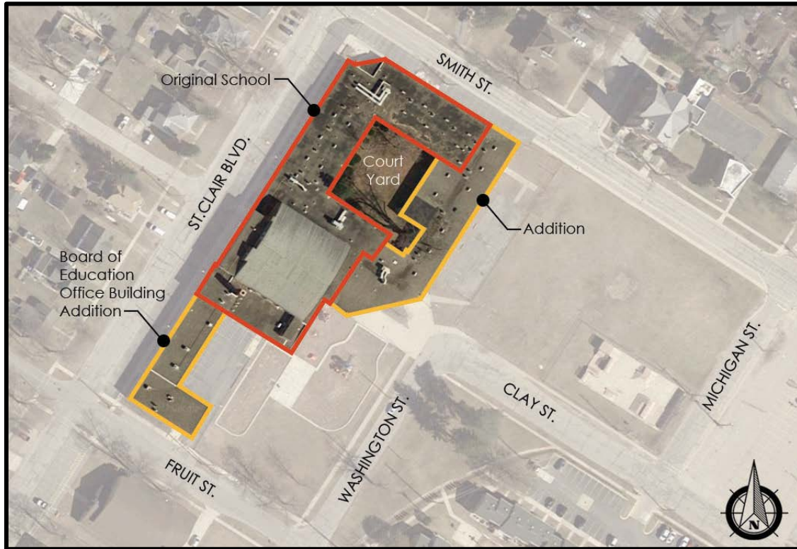
Figure 7: Building Roof Plan & Construction Phasing
